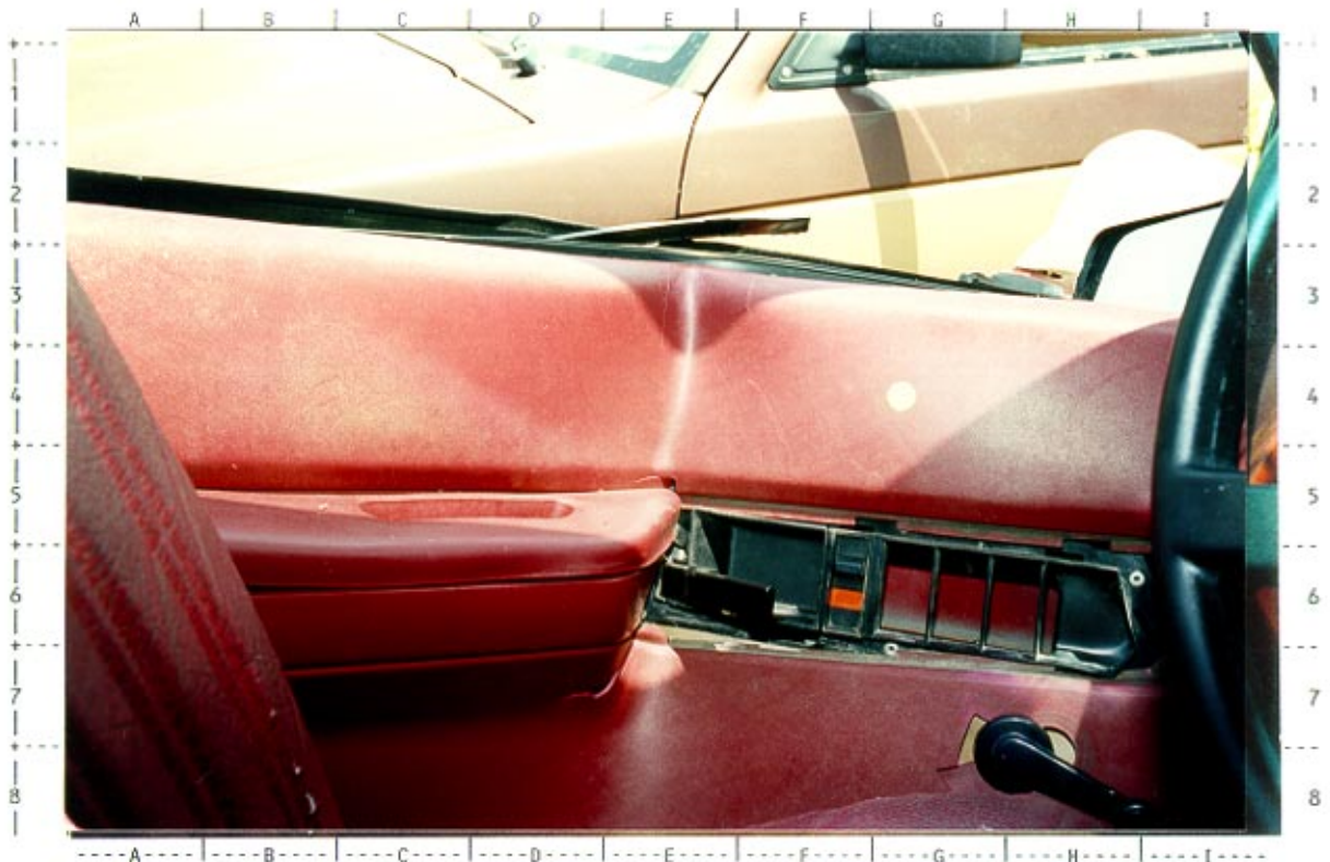
# 87 -- Close-up of probable contact to 1988 Chevrolet pickup's left door panel
